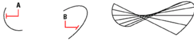
Select the first (A) and second (B) defining entities. The resulting ruled surface mesh.
